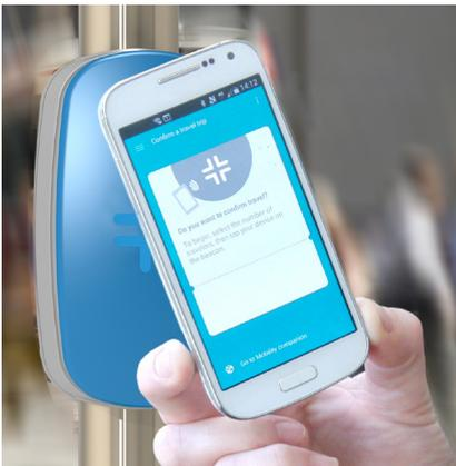
This breakthrough universal system is compatible with all mobile phone operators, is easy to install and offers the same security guarantees as conventional contactless ticketing. Commuters can use their Near Field Communication (NFC)-enabled smartphone on trains, buses, trams and any service that is equipped with Seamless<sup>®</sup> tags.
